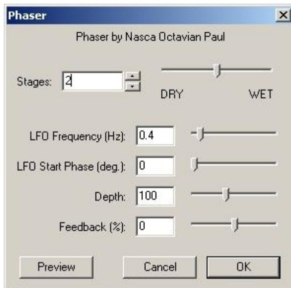
It is used in order to change the timbres of instruments (or of the human voice) in time, by using oscillators that change frequencies, and results in a change of the timbre colour in time.
