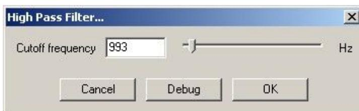
It cuts off (removes) all the frequencies under a chosen threshold. It is used to listen only to the high frequencies of an audio material or in order to remove low frequencies.
