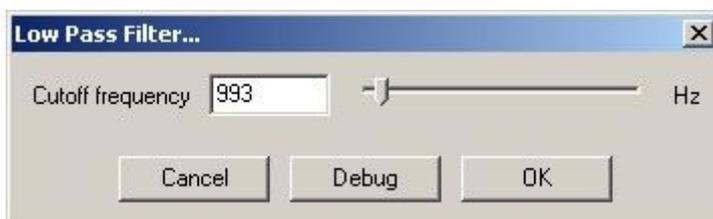
It cuts off (removes) all the frequencies over a chosen threshold. It is used to listen only to the low frequencies of an audio material or in order to remove high frequencies.
